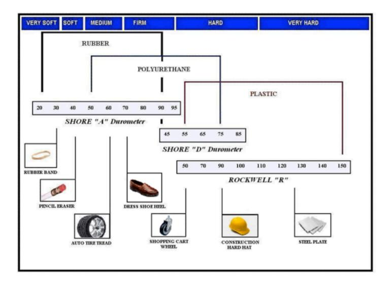
**Durometer** is typically used as a measure of hardness in polymers, elastomers, and rubbers. Hardness may be defined as a material's resistance to permanent indentation. The durometer scale was defined by Albert F. Shore, who developed a measurement device to measure **Shore hardness**, called a durometer in the 1920s. The term durometer is often used to refer to the measurement, as well as the instrument itself.
